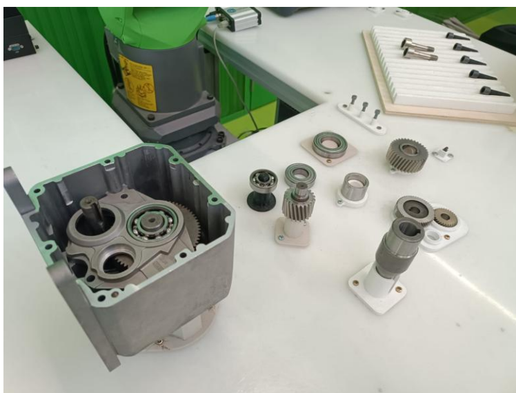
FIGURE 9: ASSEMBLY OF GEARBOX COMPONENTS.
